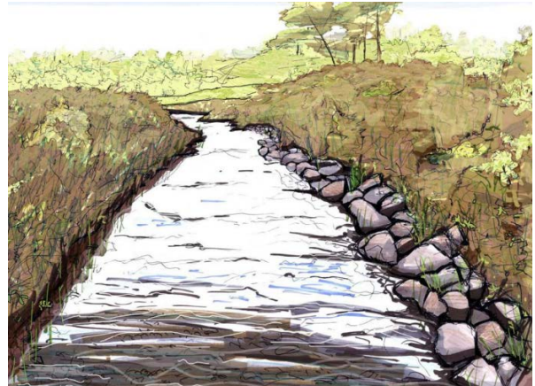
C. Bank armoring & restored vegetation
