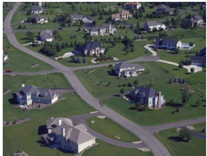
Lawn covers about 40% of the District. Compared to native forests and prairies, they shed a significant amount of stormwater and have greatly reduced stormwater infiltration.
